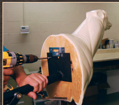
Permanently secured by screws through stand and into form backboard.
